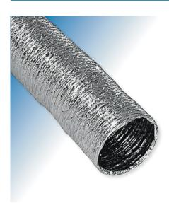
Polyaire Metallized Core fire rated flexible duct is manufactured from metallized Mylar and clear Mylar substrates, incorporating totally encapsulated helically wound spring wire. Bonded with a fire retardant and slip resistant dry deposit adhesive, this duct construction ensures a long life span in all ambient conditions.
